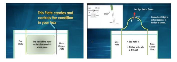
Connect the plates together with a copper wire. Cut the wire and insert a LED (red of green). The LED acts as a resistance to the flow of current between the plates.
